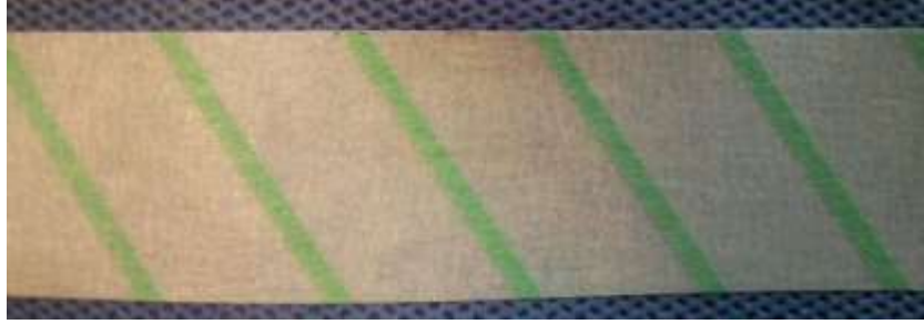
Starting color of unexposed indicator of ITSG-tape:
