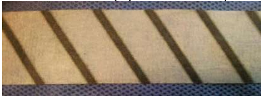
End colors of correctly exposed indicator of ITSG-tape:
