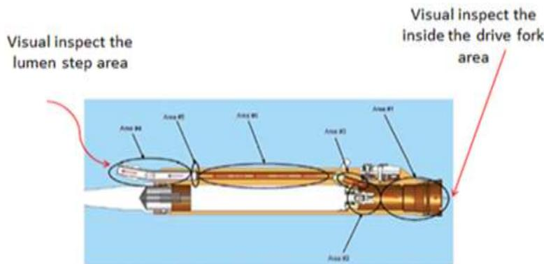
IFU Support for using a Flexible Inspection Scope:
