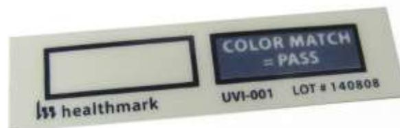
The intensity of the UV light source that we had for our internal tests was 7200  $\mu\text{W}/\text{cm}^2$  at one foot, making the UV dose 432  $\text{mJ}/\text{cm}^2$ .
