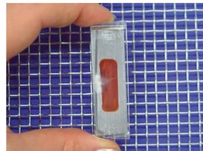
**The type of soil left on the TOSI after being run through a washer indicates potential problems with the equipment.**
