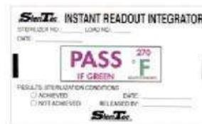
After the sterilizer has run its cycle, drying time is about 30 minutes that is recommended after the load is complete before removing it from the sterilizer. The biological indicator should then be put into the incubator and read at the appropriate time. Section C.8 Test results states, “All test BIs must be negative and all test CIs must reach their endpoint. Any results to the contrary must investigated”. Record all load information with all sterilization parameters met including
